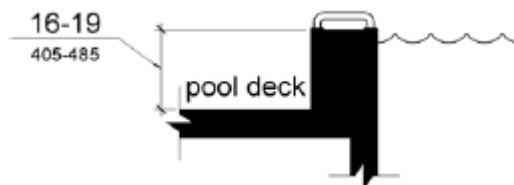
Figure 1009.4.2 Transfer Wall Height
